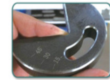
Chamfering effect chamfering depth 0-3mm adjustable
